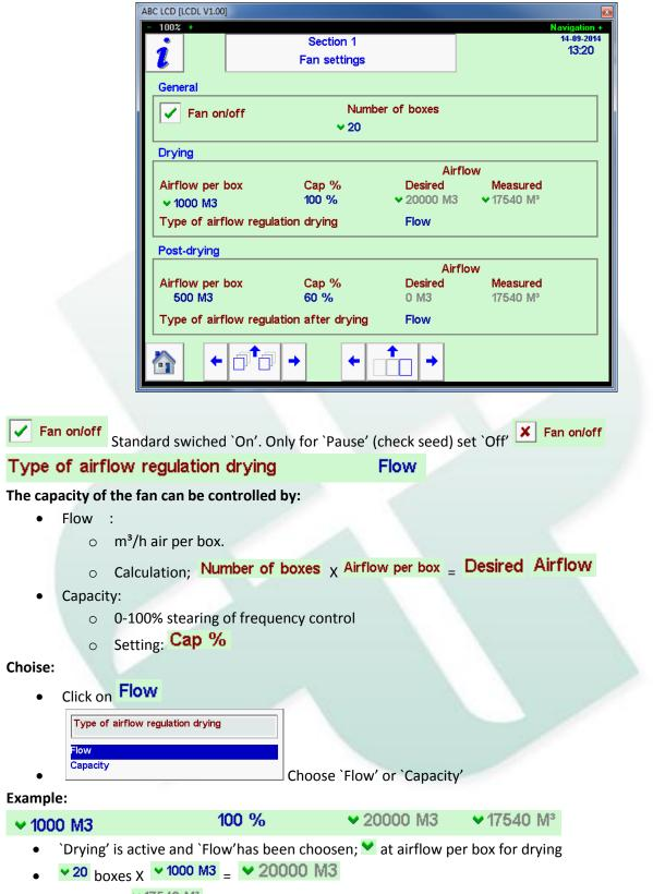
• Measured <sup>▼17540 M³</sup>, but stearing to +/- 200 M3 of desired airflow.
