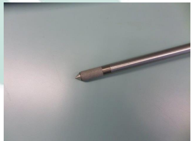
Measurement of RH+T° at the tip of the sensor
