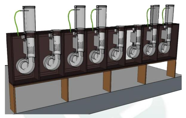
A small high pressure fan blows air through an electrical heater into the tube to make the seed fluid.
