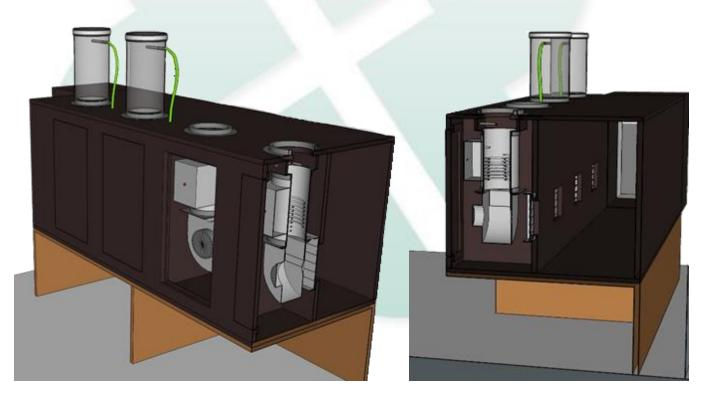
Air will be extracted from a central duct at the back; fresh and dry air to prevent recycling of damp air.
