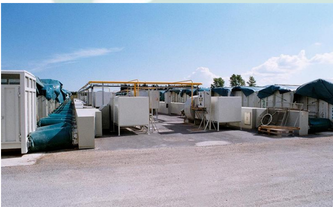
Example of drying process in containers. Airflow would be automatically controlled and on the amount of containers.
