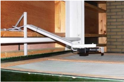
Sensor in the outgoing airflow of a drying box. Measuring T° and RH per section (box, tray, container).
