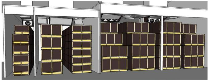
Depending on the needs and use, the lay-out and measurements of the cells are determined: 1 or more row of boxes per cell or 1 large cell with drying on 2 sides, 3-4-5-6 boxes stacked high. Volumes up to 30 or 40 m<sup>3</sup> per row are possible.
