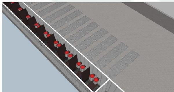
The drying can start directly when a row is filled with boxes. In this row the seed is gradually warmed with increasingly warmer air;
