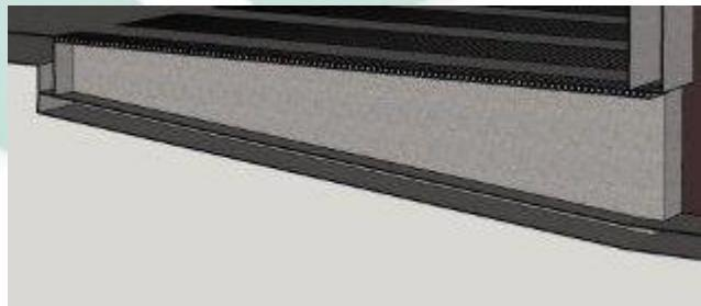
By measuring the air condition of the air from the seed, it can be determined if the seed in the row begins to dry. If that occurs, the moisture will be discharged with less and less air. The slide can therefore gradually close. Because of this an unfavorable row will eventually get enough air to dry too.
