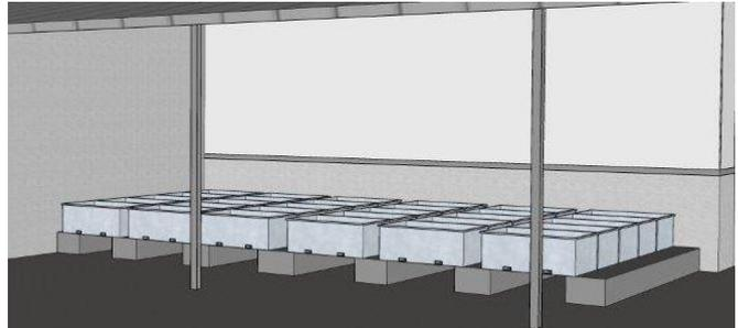
Box drying in above-ground ducts with 'skids'
