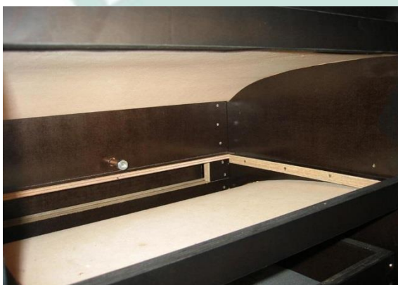
Air-inlet and air guidance per drawer.
