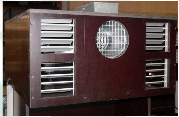
Extracting unit including heater and valves.
