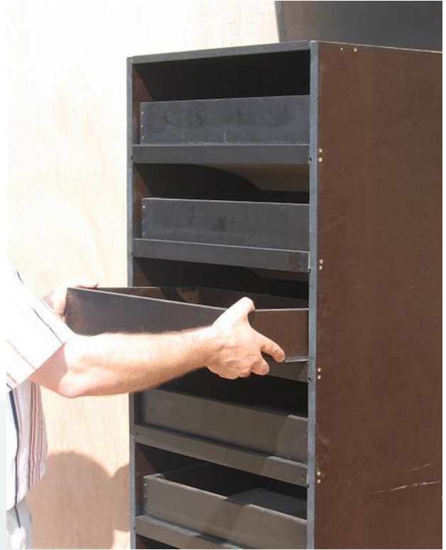
Air-inlet opens when drawer is being placed.
