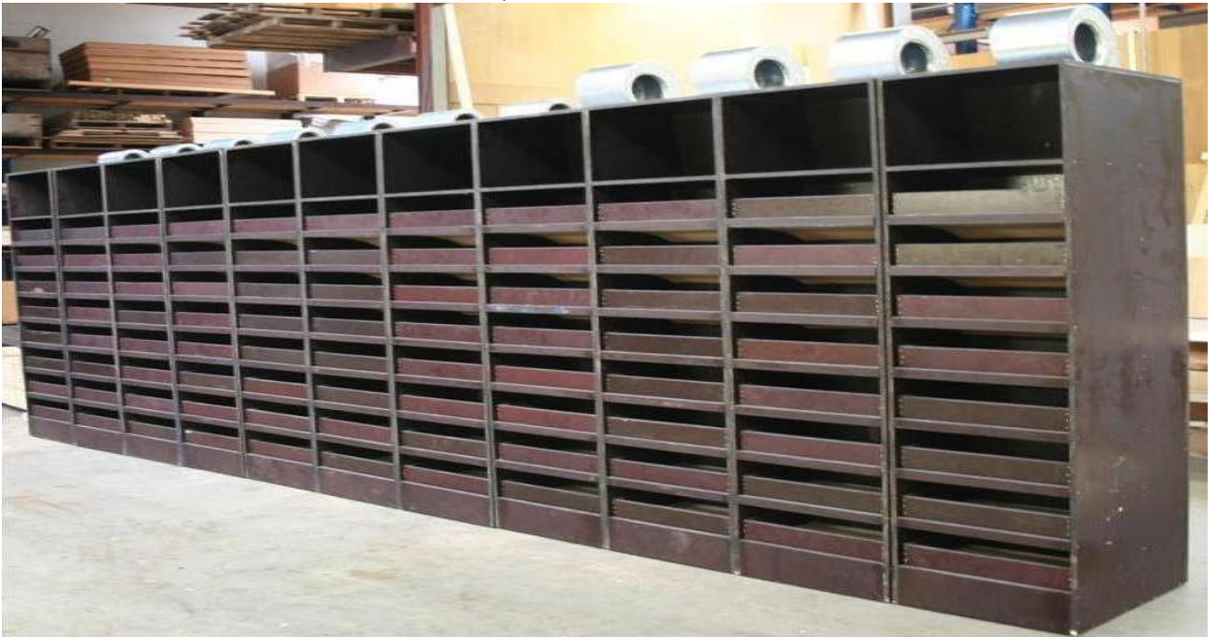
Drying / ventilation units for drawers.
