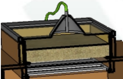
The T°+RH measurement sensor (c) has been mounted onto the cover grid using a funnel, to measure the air condition from the seed.
