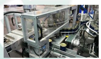
The can filling and seaming machine was equipped with new pneumatics and the existing line supply and discharge was optimized.
