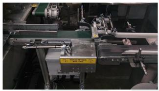
The check weighing has changed from belt weighing to static weighing: more accuracy and less sensitivity to failures.
