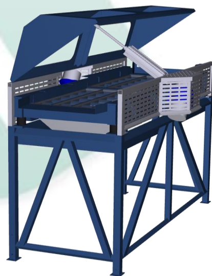
Small flats screen sizer 400 mm wide for 3 fractions. Used for laboratory seed cleaning and pellets.
