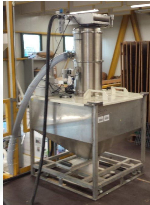
Continues seed supply by vacuum systems on a hopper bin.
