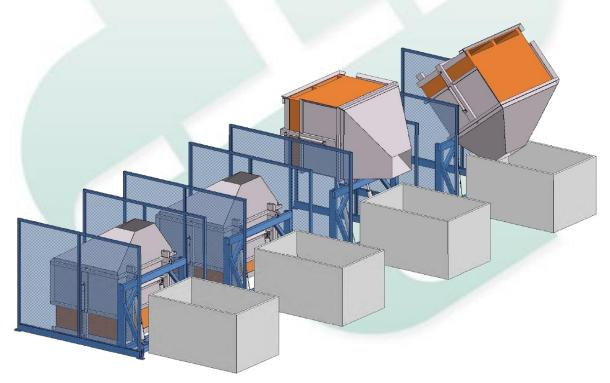
Here you see the inverting process. The outflow can be adjusted if desired. Can be equipped with a dosing slide or outflow opening for the connection with the vacuum transport system.
