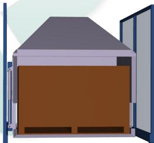
The sides are provided with cylinders to be able to lift the box to close the space between the funnel.
