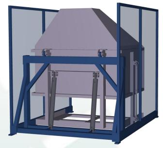
The cylinders are used to invert the top of the inverting yoke.
