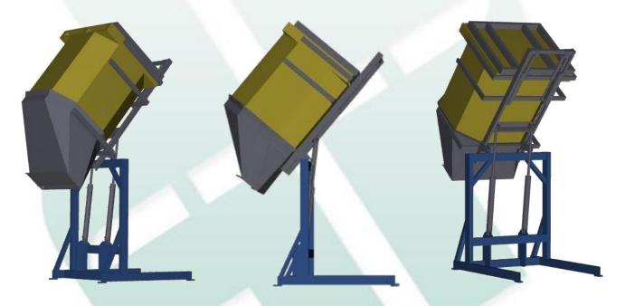
Cylinders ensure that the octabin will turn over. The funnel outlet reaches the box, elevator or bunker.
