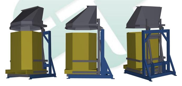
The octabin with pallet is placed in the inverter. The funnel is lifted to have enough space to place the octabin.
