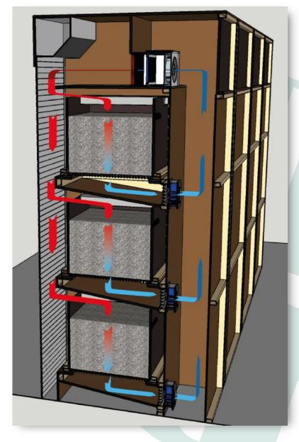
A high-pressure fan has been installed for each box. The air volume can thus be configured per box to match the quantity and type of the seed.
