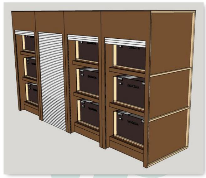
The conditioned box dryer is a closed installation with which the seed is dried to the desired moisture content at the desired air condition. This by using dried and cooled air. The boxes are placed separatedly from each other in an air distribution system. Which ensures that the air is sucked through the seed. The air distribution system is located in a closed casing so that the seed can be dried regardless of the outside conditions.
