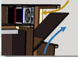
The picture above shows an option to remove humid air to the outside and to draw in drier (outside) air. In the case of moist seed, the drying time is thus greatly reduced. When the air from the seed becomes drier than the outside air, this air will automatically be used in the drying process.
