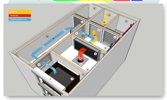
When the air from the product is drier than the outside air, this dry air is recirculated.
