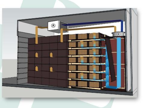
Humidifier in closed cell with internal circulation.
